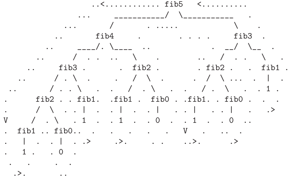
Figure 1.5: The tree-recursive process generated in computing (fib 5).
