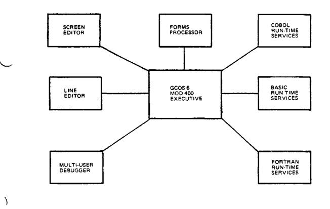
Figure 1-1. Application Development Components
